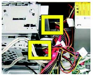
Figure 2-52 Disconnecting the power cable
